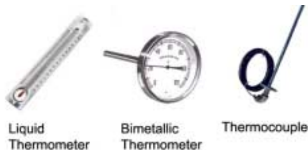
Figure 4-1 Temperature Measuring Instruments
